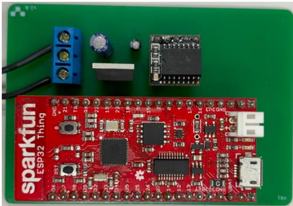
Figure 4.25. The master prototype is designed with own Real-time clock for ensuring the restoration of the data integrity by labeling with data-time components
